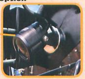
Optional camera located on the right side of the TrucKat allows the operator to view the cutting head in operation while facing forward and steering vehicle.
